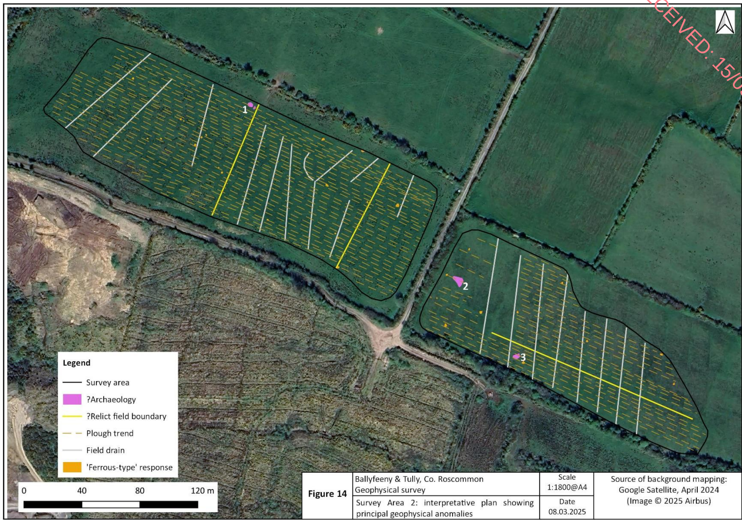
Figure 14. Survey Area 2: interpretative plan showing principal geophysical anomalies.
