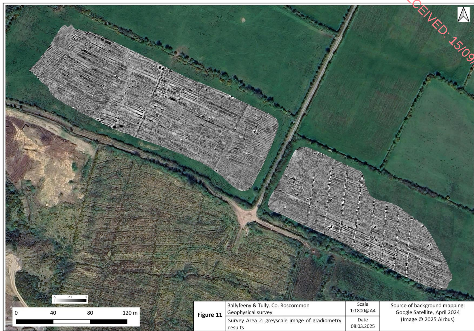
Figure 11. Survey Area 2: greyscale image of gradiometry results.
