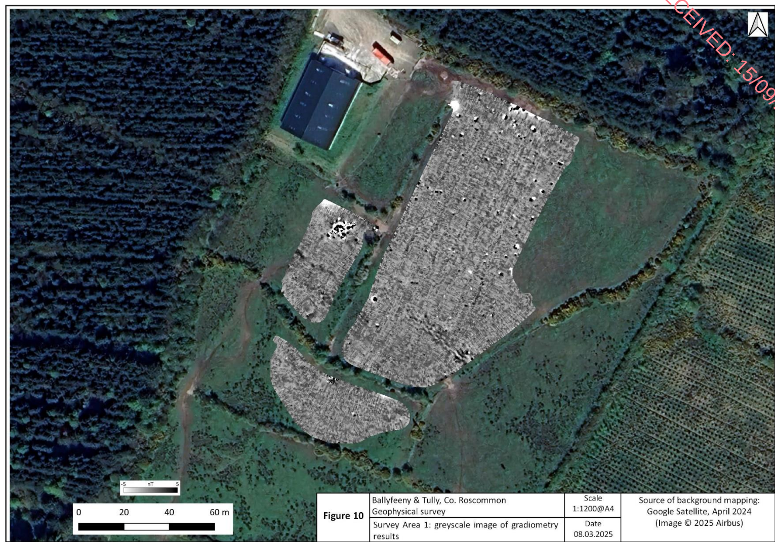
Figure 10. Survey Area 1: greyscale image of gradiometry results.
